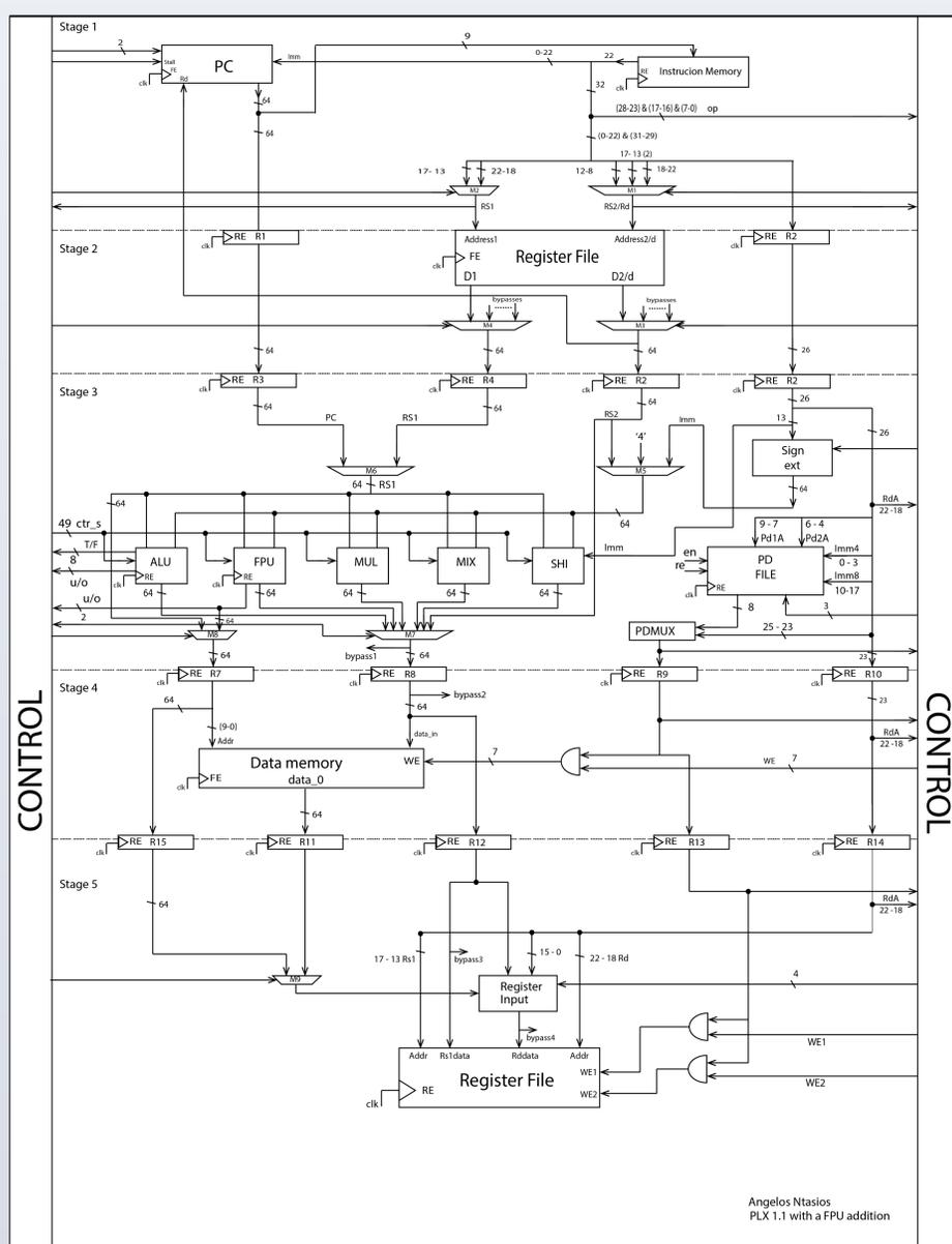
Figure 1. The Processor RTL Schematic
