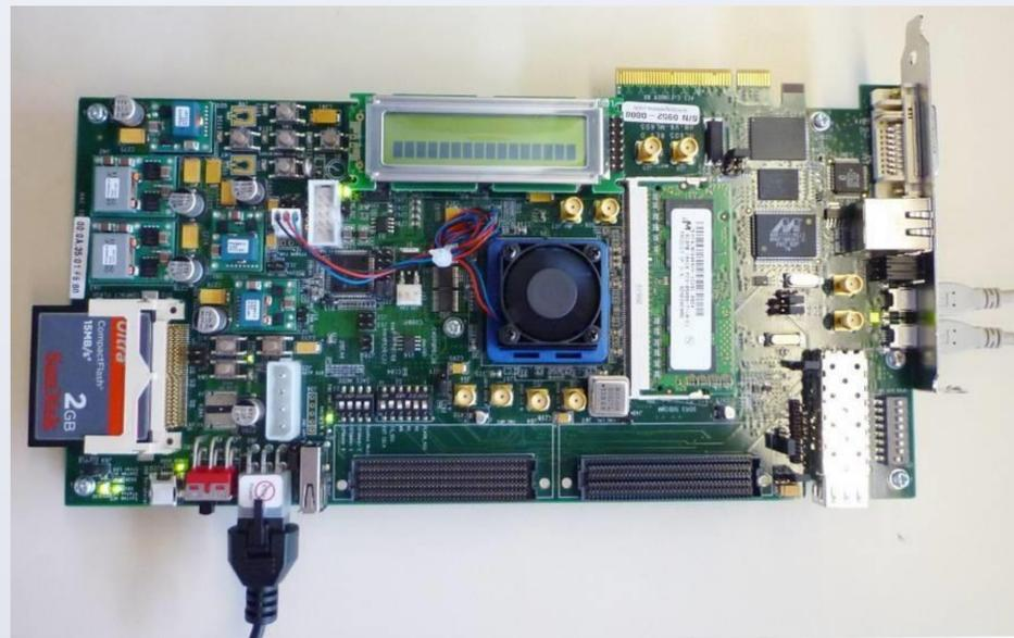
The Xilinx Virtex 6 ML605 FPGA Board that was used for the implementation
